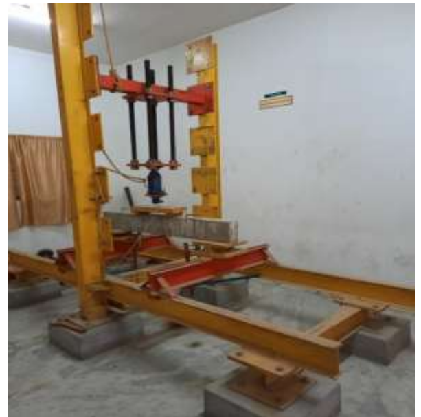
Fig (2) Simulations of Hinged end conditions for the specimen during the testing.
