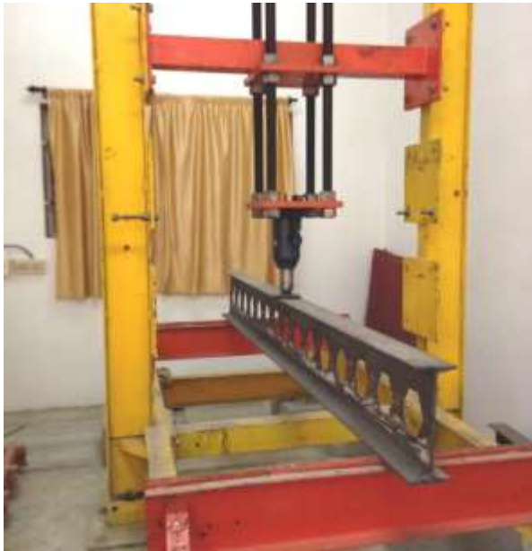
Fig (1) Reaction Frame with Castellated Beam during experiment (200 KN)
