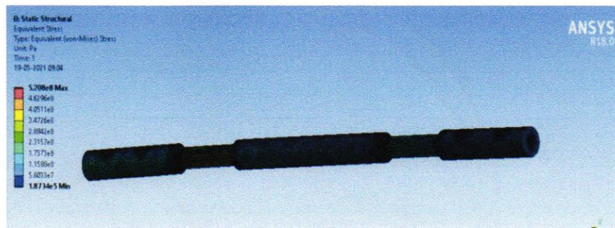
Figure 5.5.32: Aluminum beam subjected to torque of 6 Nm and axial load of 150 N
