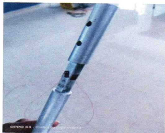
Figure 6.2: Fabricated Model with strain gauge
