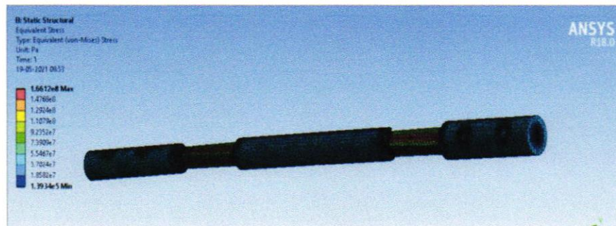
Figure 5.5.25: Steel beam subjected to torque of 10 Nm and axial load of 5 N
