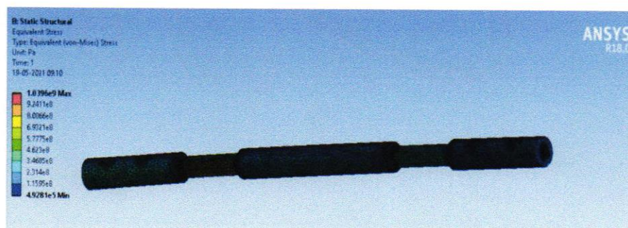
Figure 5.5.35: Aluminum beam subjected to torque of 10 Nm and axial load of 150 N
