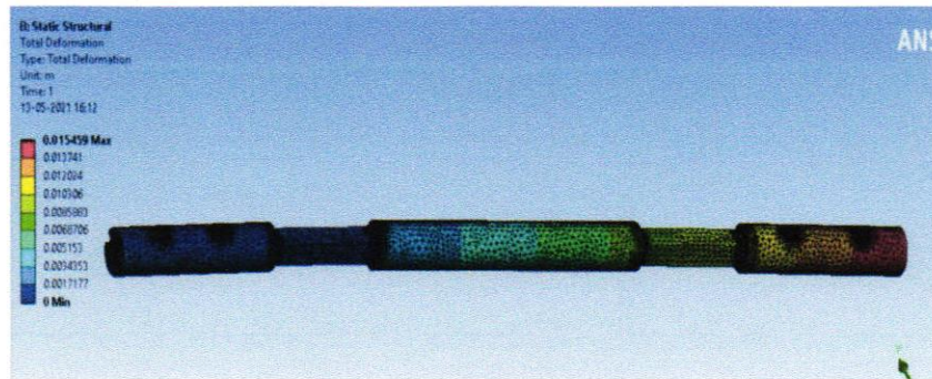
Figure 5.4.3: Steel Loaded under axial load of 5 N and longitudinal load of 300 N
