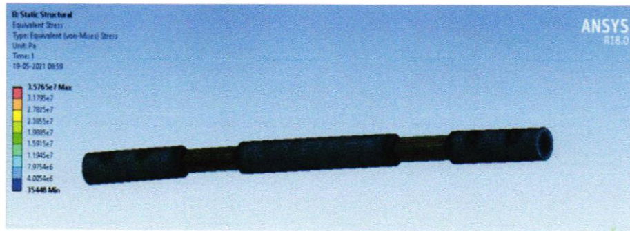
Figure 5.5.28: Aluminum beam subjected to torque of 2 Nm and axial load of 5 N
