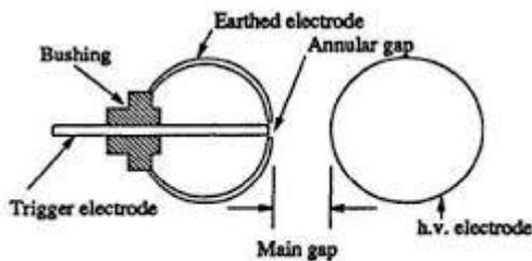
Figure:3.26 (a) Trigatron gap
