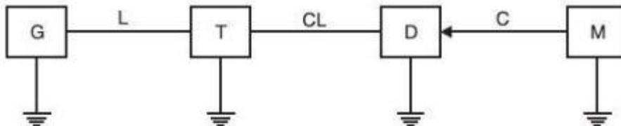
Figure: 4.7 Basic voltage testing circuit
