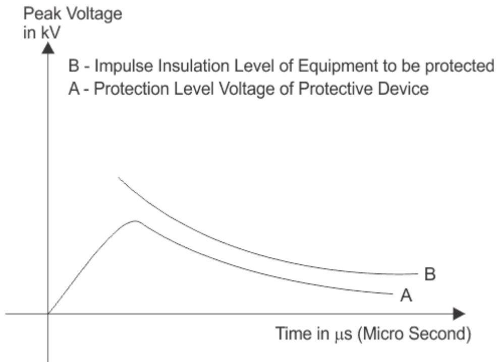
Voltage - Time Curved Used for Insulation Coordination
